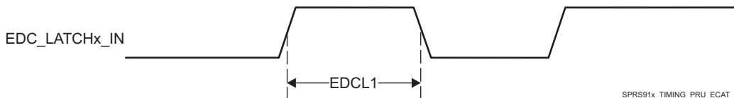
Figure 5-120. PRU-ICSS ECAT LATCHx_IN Timing
