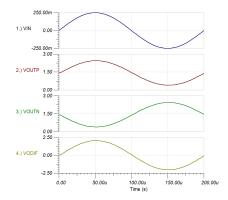
Figure 2. Differential Output Voltage
