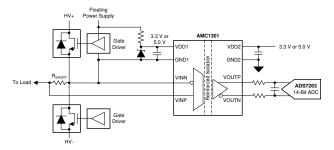
Figure 1. AMC1301 Functional Block Diagram
