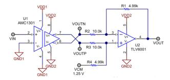
Figure 5. Scaled Differential to Single-Ended Output
