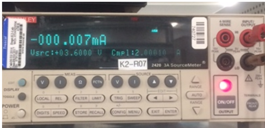
Figure 6. Reduced Leakage Current Confirmed with Keithley Sourcemeter
