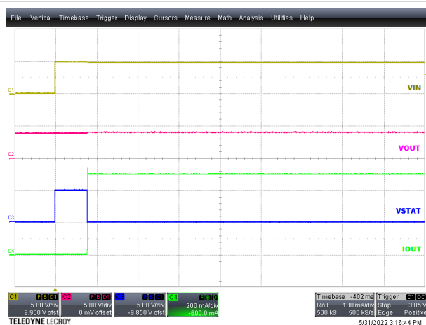
Figure 8-2. Power Up with Battery
