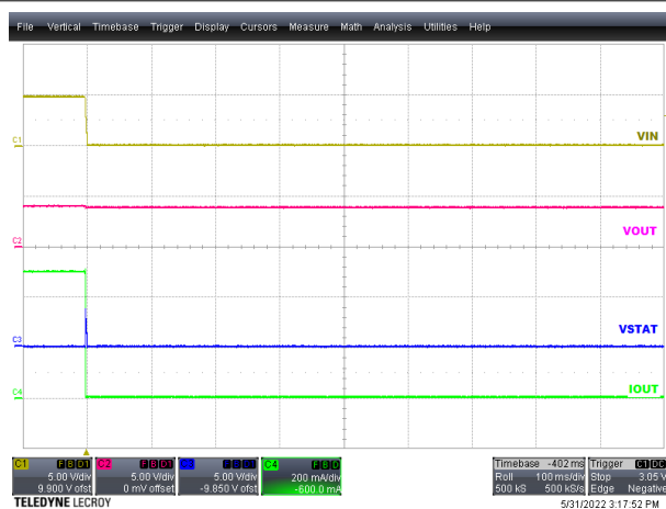
Figure 8-2. Power Up with Battery
