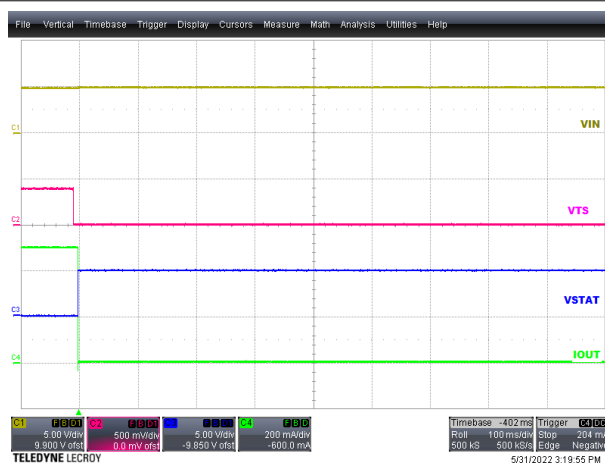
Figure 8-3. Power Up without Battery
