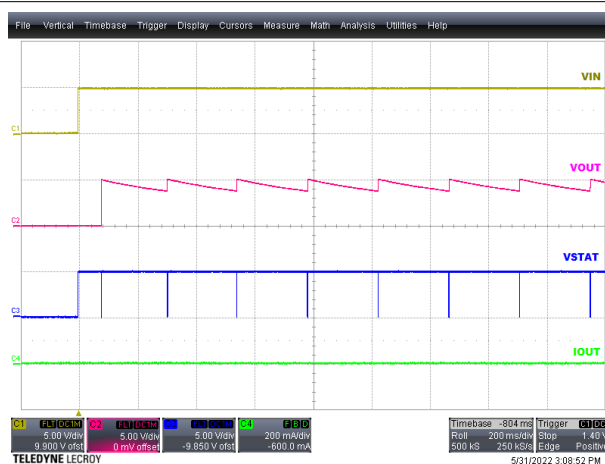
Figure 8-3. Power Up without Battery
