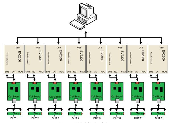
Figure 9. Multi-Station Setup
