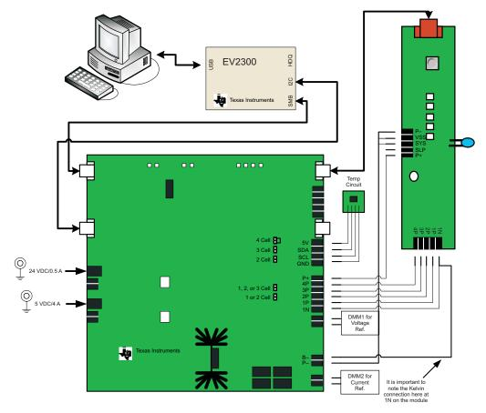
The bqMTester from Texas Instruments is designed to calibrate and program electronic smart battery modules based on the bq20zXX and future advanced battery gas gauges. The bqMtester consists of a software suite, a maximum of 12 calibration boards (HPA169) and an equal number of communication boards (EV2300 – purchased separately).
