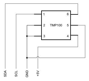
Figure 7. External Temperature Sensor Connection
