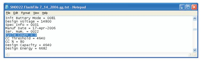
Figure 3. Cycle Count Modification in GG File Using Notepad
