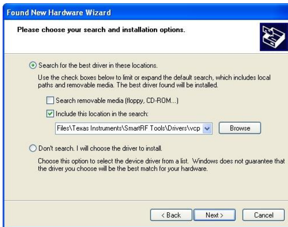
Figure 1 – Install virtual COM port USB driver using the Windows Hardware Wizard
