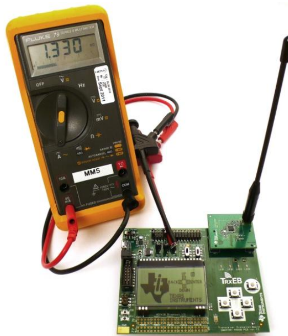
Figure 19 – Current measurement setup
