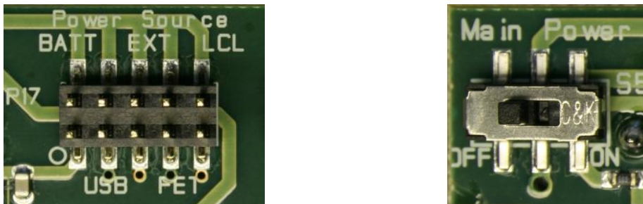
Figure 6 – Main power selection header (P17) and power switch (P5)
