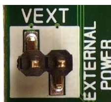
Figure 11 – TrxEB rev. 1.7.0 external power supply header (P1)
