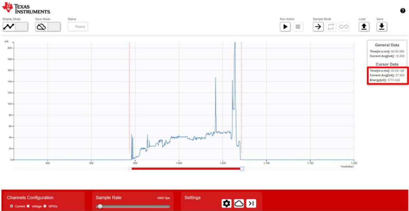
Figure 16. Average Current Measurement With IMETER-BOOST Device
