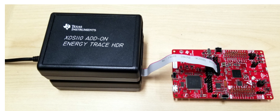
Figure 27. CC3220 Device Test Setup With XDS110 System
