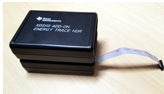
Figure 19. XDS110 Probe and ETHDR System
