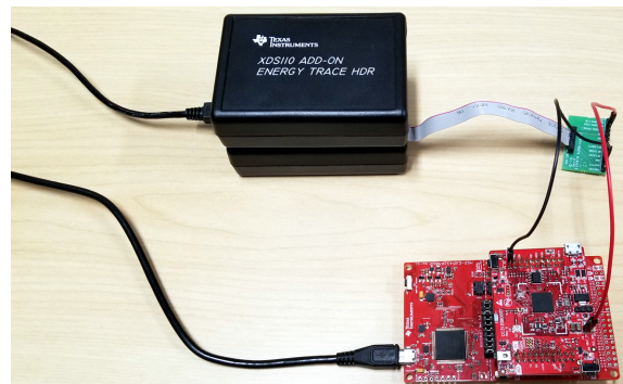
Figure 26. CC3120 Device Test Setup With XDS110 System
