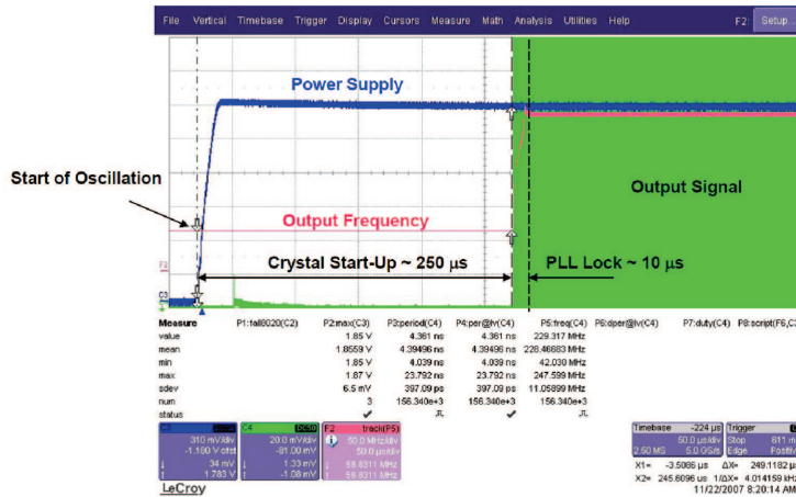
Figure 17. Crystal Oscillator Start-Up vs PLL Lock Time
