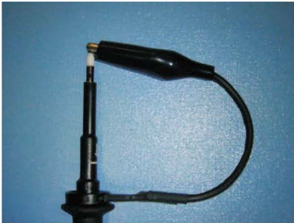
Figure 5. Ringing Voltage Pick-up by 3-Inch Ground Wire
