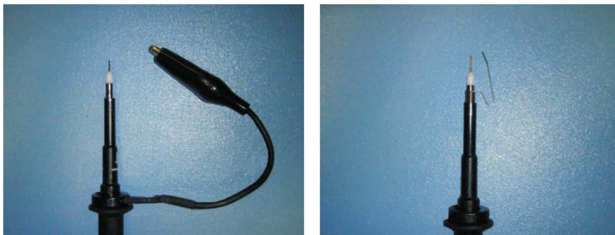
Figure 7. Oscilloscope Probe Comparison: Typical 4-Inch Wire (Left) Versus Small Length Wire (Right)
