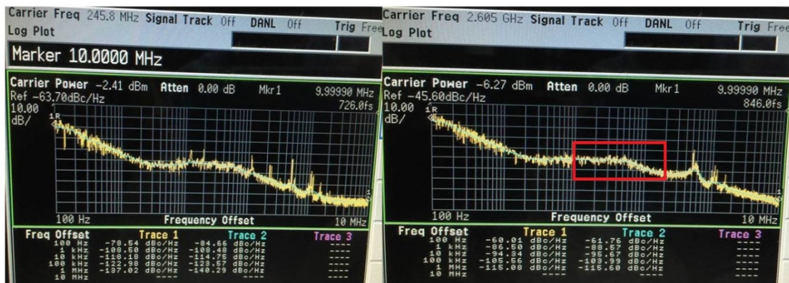
Figure 5. PLL Reference Clock Phase Noise (Left), and Normal DAC Output Phase Noise at 2605 MHz at 5-MHz PLL Loop Bandwidth (Right)
