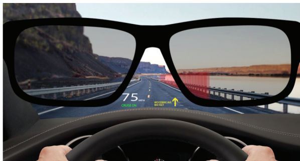
Figure 13. When using DLP technology, polarized sunglasses have no effect on HUD images
