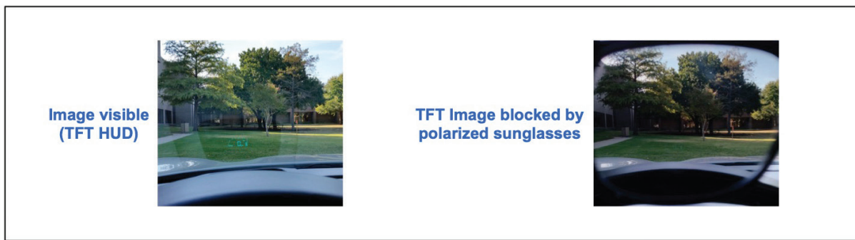
Figure 12 . While polarized sunglasses reduce glare, they can also unfortunately filter out TFT-created HUD images
