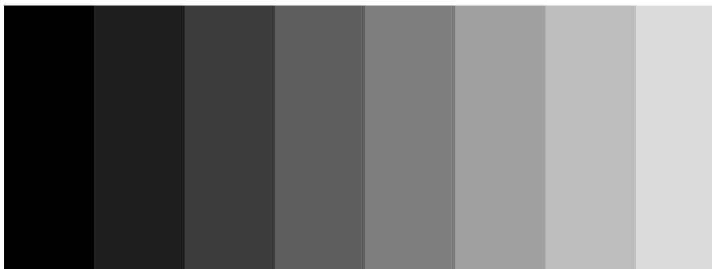
Figure 3-10. Example of Fixed Step Horizontal Ramp Test Pattern
