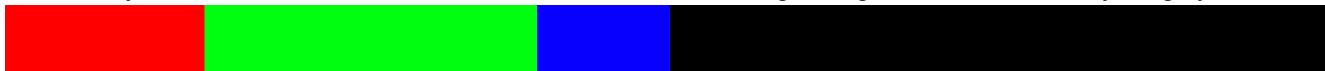
Figure 3-3. Example illumination sequence with one color cycle per LED, and 50% dark time
