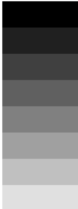
Figure 6. Example of Fixed Step Vertical Ramp Test Pattern
