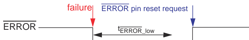
Figure 21-115. \overline{\text{ERROR}} Pin Timing - Example 3
