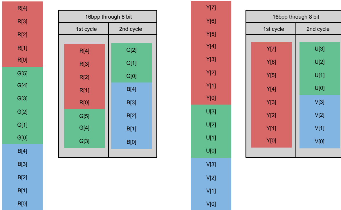
Figure 6. YUV422 Output Through TDM
