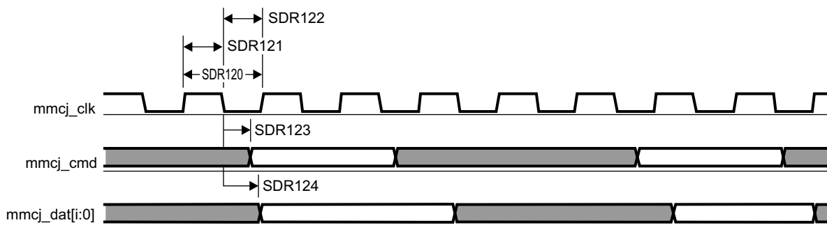
Figure 7-88. MMC/SD/SDIOj in - SDR12 - Transmitter Mode
