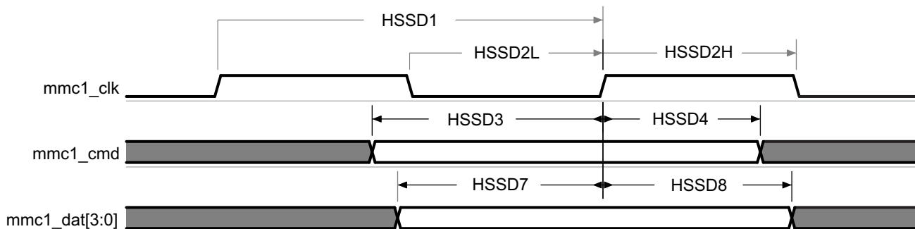
Figure 7-64. MMC/SD/SDIO in - High Speed - Receiver Mode
