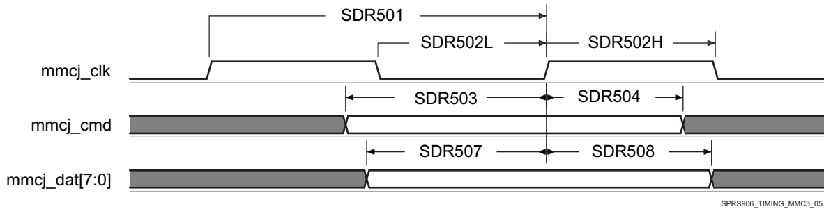
Figure 5-107. MMC/SD/SDIOj in - High Speed SDR50 - Receiver Mode
