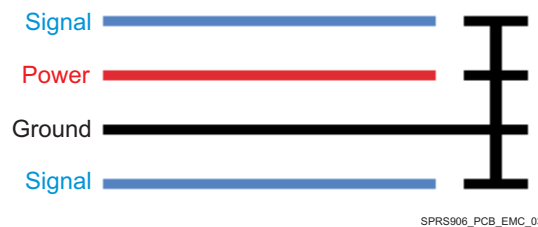
Figure 7-13. Guard Ring Routing
