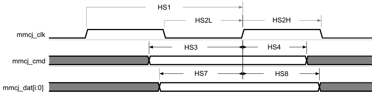
Figure 5-101. MMC/SD/SDIOj in - High Speed 3.3V Signaling - Receiver Mode
