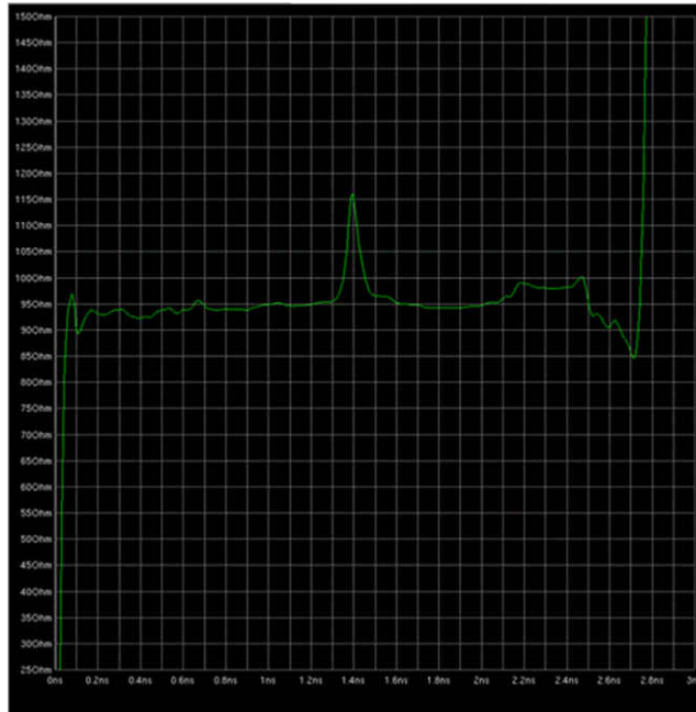
Figure 3-1. TDR Plot Example With Impedance Mismatch
