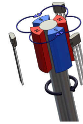
Figure 6. Rotor Position Using TO-92 Hall Sensor
