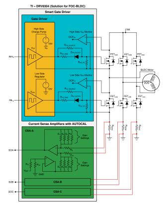
Figure 1. TI Smart Gate Driver for FOC Implementation
