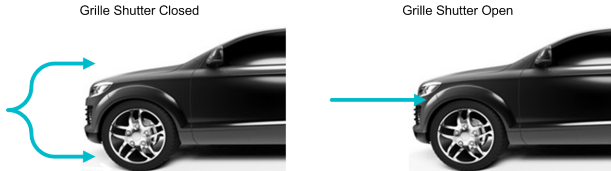
Figure 1. Air Flow With Grille Shutter Open and Closed
