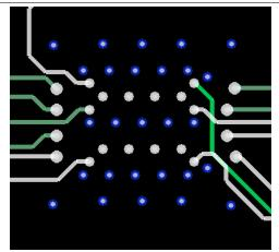
Figure 26. Internal Low-Speed Signal Layers (Pin A1 is Top-Left)
