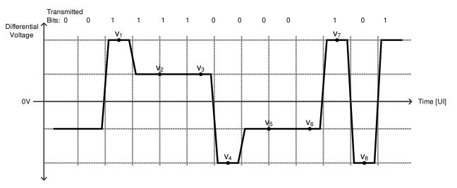
Figure 8. Conceptual FIR Waveform With Postcursor Only
