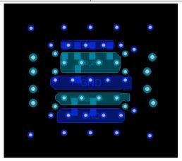
Figure 28. Bottom Layer (Pin A1 is Top-Left)
