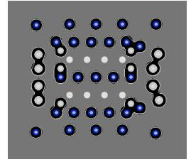
Figure 27. VDD Layer (Pin A1 is Top-Left)
