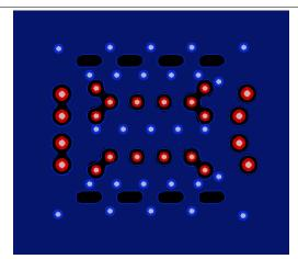
Figure 25. Layer 1 GND (Pin A1 is Top-Left)
