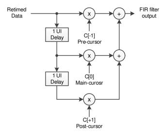
Figure 7. FIR Filter Functional Model
