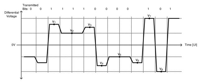
Figure 10. Conceptual FIR Waveform With Both Precursor and Postcursor
