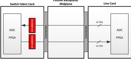
Figure 20. Backplane/Mid-Plane Application Block Diagram (Top: Recommended Placement; Bottom: Placement With Both Retimers on the Same board)
