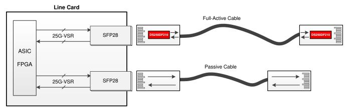
Figure 18. Active Cable Application Block Diagram
