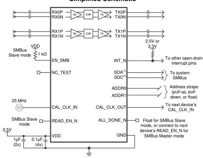
(1) SMBus signals need to be pulled up elsewhere in the system
