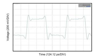
Figure 23. DS250DF210 FIR Transmit Equalization While Operating at 25.78125 Gbps
