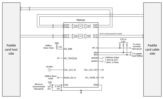
Figure 19. Full-Active Cable Application Schematic
