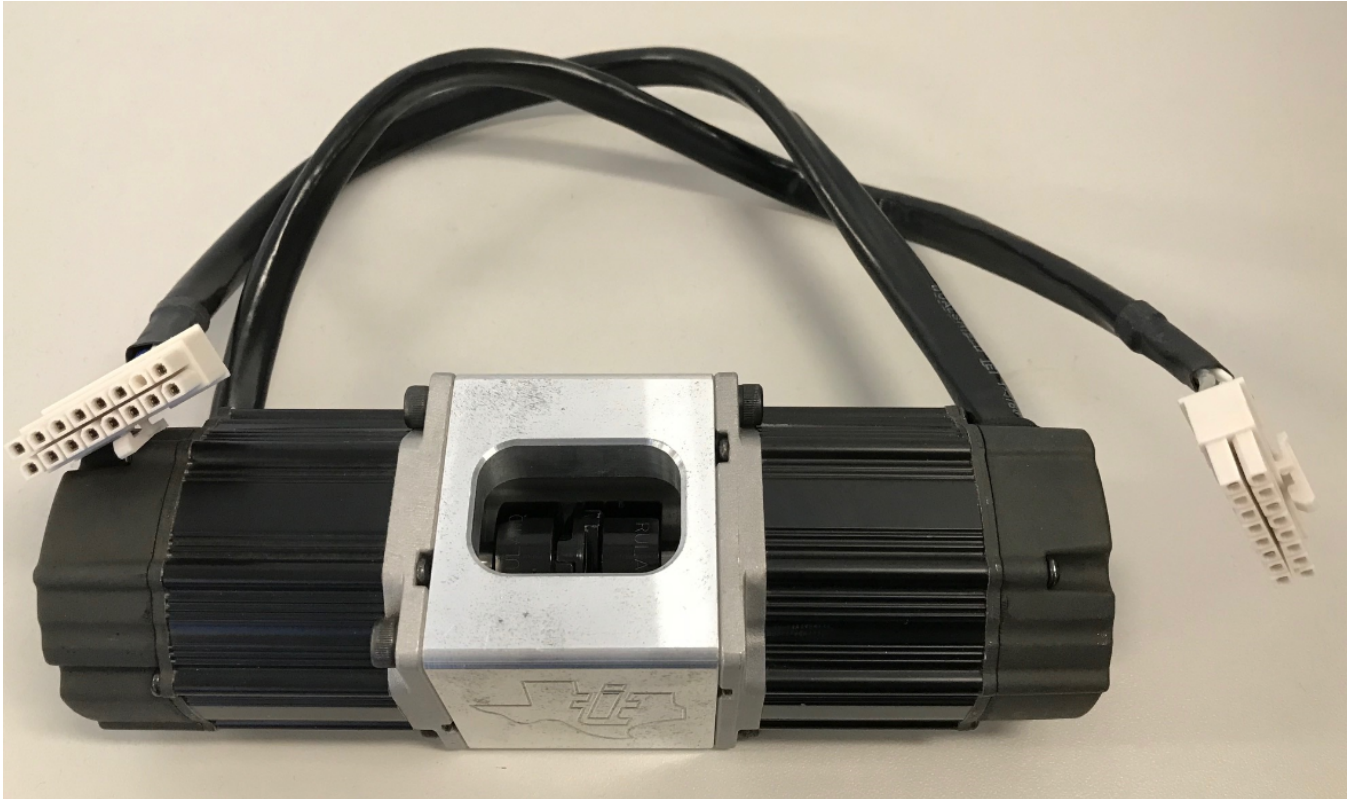
Figure 9. Two Motor Dyno Set
