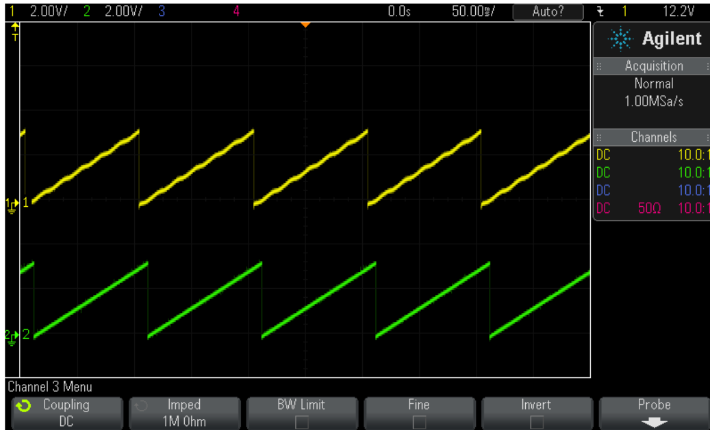
Figure 14. Scope Plot of Reference Angle and Rotor Position
