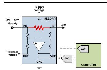
Figure 2. Integrating The Current Sensing Resistor
