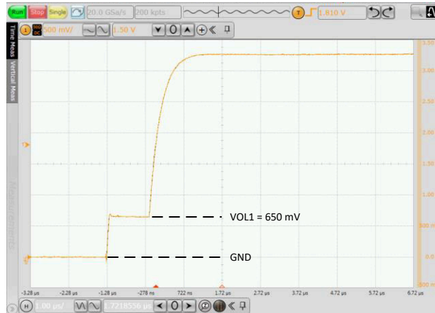
Figure 9-7. Side 1 ISO1640: Low-to-High Transition
