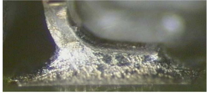
Figure 13. Group 1B, NiPdAu Finish, Stored in Tubes, 96-h Exposure
