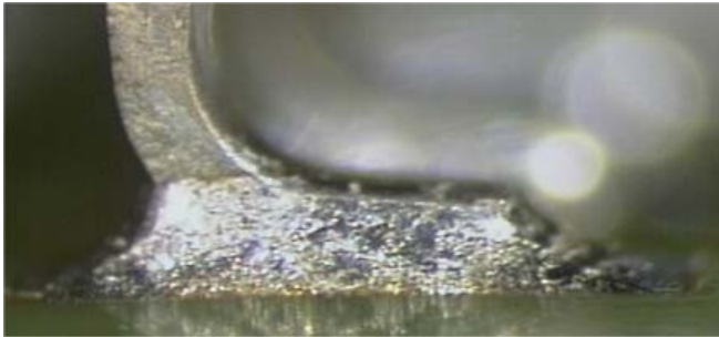
Figure 14. Group 2A, NiPdAu Finish, Stored Loose, 96-h Exposure
