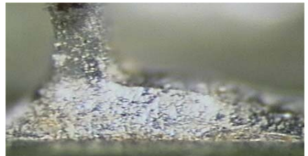
Figure 23. Group 6B, NiPdAu-Ag Finish, Stored in Tubes, 96-h Exposure
