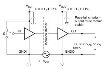
A.  $C_L = 15pF$  and includes instrumentation and fixture capacitance within ±20%.
