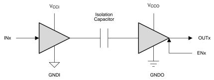
V<sub>CCI</sub> and GNDI are supply and ground connections respectively for the input channels.
