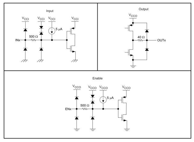
Figure 14. Device I/O Schematics
