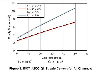
Figure 1. ISO7142CC-Q1 Supply Current for All Channels vs **Data Rate**
