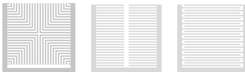
Figure 2. Examples of Effective Coil Shielding Structures
