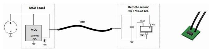
Figure 3. TMAG5124 Two-Wire Connection and Small PCB Implementation
