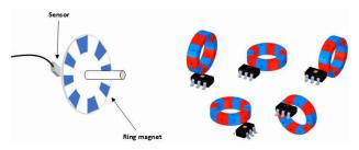
Figure 1. Rotary Encoding Using Ring Magnets, and Various Sensor Placements
