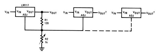
\*All outputs within ±100 mV †Minimum load—10 mA
