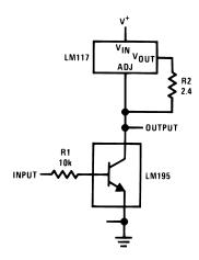
Figure 29. High Gain Amplifier
