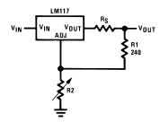
Figure 17. Regulator with Line Resistance in Output Lead
