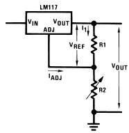
Since the  $100\mu A$  current from the adjustment terminal represents an error term, the LM117 was designed to minimize  $I_{ADJ}$  and make it very constant with line and load changes. To do this, all quiescent operating current is returned to the output establishing a minimum load current requirement. If there is insufficient load on the output, the output will rise.
