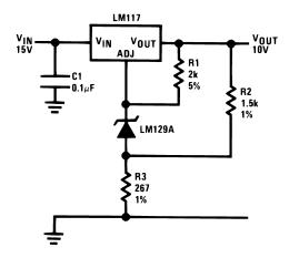
Figure 22. High Stability 10V Regulator
