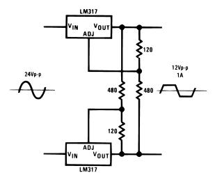
Figure 36. AC Voltage Regulator
