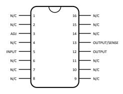
For the Ceramic SOIC device to function properly, the "Output" and "Output/Sense" pins must be connected on the users printed circuit board.
