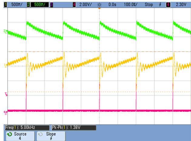
Figure 13. Load Transient Response of Positive and Negative Output Rail With Symmetrical Loads (1A)
