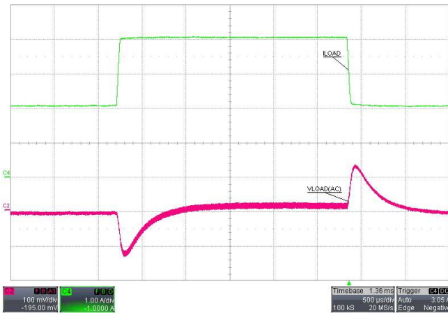
Figure 6. Load Step: I_{LOAD} 2A to 4A, V_{SUPPLY} = 18V
