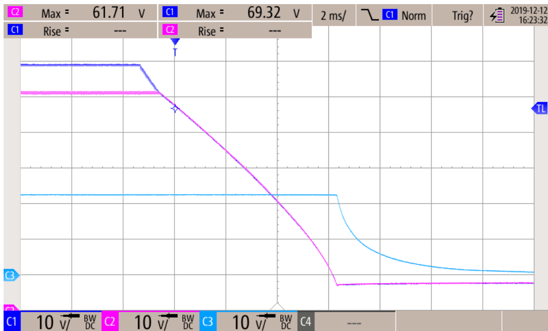
Figure 23. Turn-off Behavior From 70 V to 0 V (EVM Loaded With a 220-Ω Resistor)
