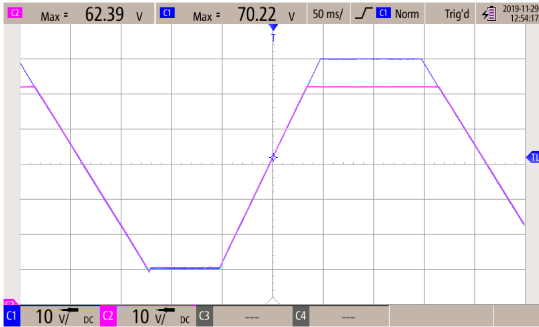
Figure 15. Waveforms for the Circuit With the TL431-Q1 Voltage Regulator (EVM Loaded With a 220-Ω Resistor)
