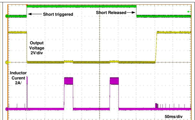
Figure 6. LM60440 Short-Circuit Transient and Recovery
