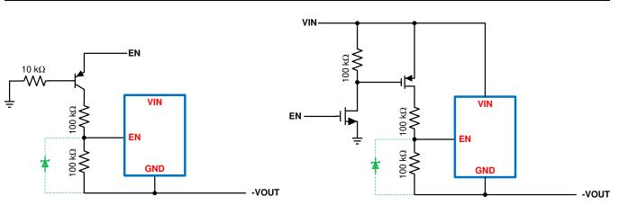
Figure 10. Enable Level Shifters
