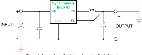
Figure 2. Converting a Buck to an Inverting Buck-Boost
