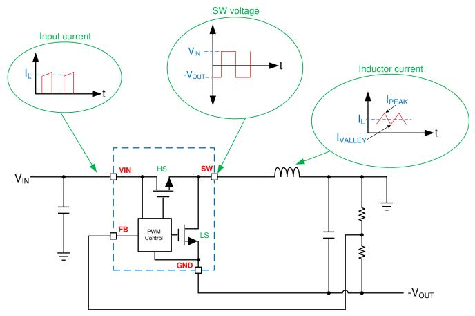
Figure 3. Inverting Buck-Boost Waveforms
