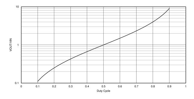
Figure 4. Conversion Ratio vs Duty Cycle
