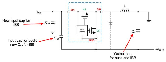
Figure 9. IBB External Components
