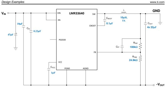
Figure 14. +12 V to -5 V, 3-A Design with the LMR33640
