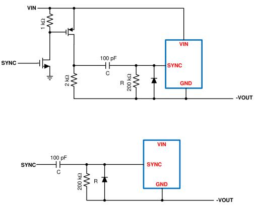
Figure 11. Synchronization Level Shifters
