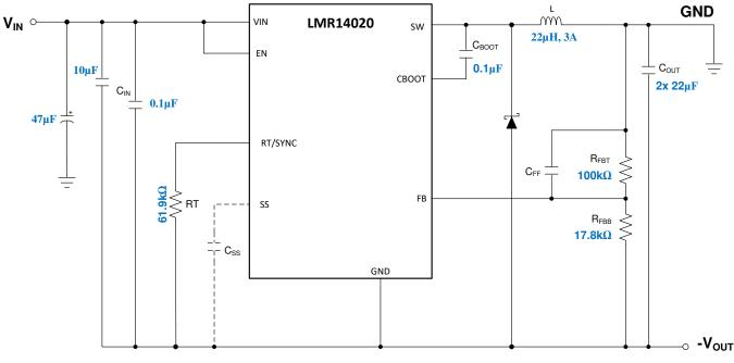
Figure 15. +5 V to -5 V, 1-A Design with the LMR14020
