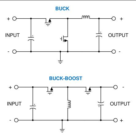
Figure 1. Comparison of Buck and Inverting Buck-Boost Topology
