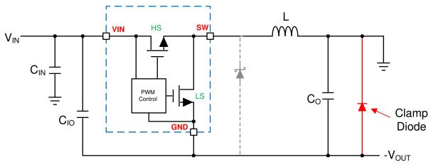
Figure 13. Output Clamp Diode
