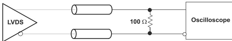
Figure 7-1. LVDS Output DC Configuration During Device Test
