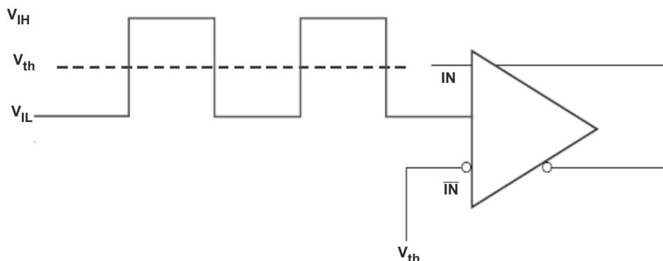
Figure 7-3. DC-Coupled LVCMOS Input During Device Test
