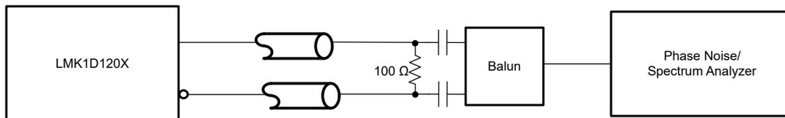
Figure 7-2. LVDS Output AC Configuration During Device Test
