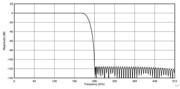
Figure 7. Magnitude Response for the ADS127L01 Wideband Filter up to  $f_{DR}$
