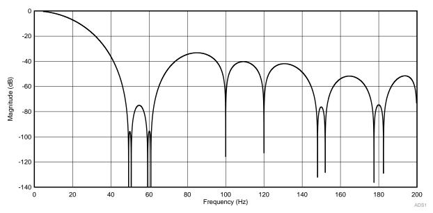
Figure 6. Magnitude Response of the ADS124S08 Digital Filter,  $f_{DR} = 20$  SPS
