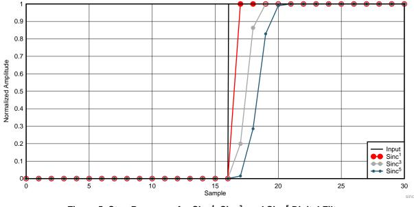
Figure 5. Step Response for Sinc<sup>1</sup>, Sinc<sup>3</sup>, and Sinc<sup>5</sup> Digital Filters
