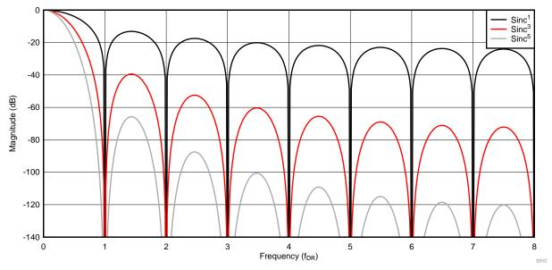
Figure 4. Frequency Response of Sinc<sup>1</sup>, Sinc<sup>3</sup>, and Sinc<sup>5</sup> Digital Filters
