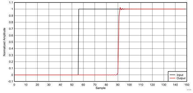
Figure 8 shows the step response of the wideband filter of the ADS127L01.
