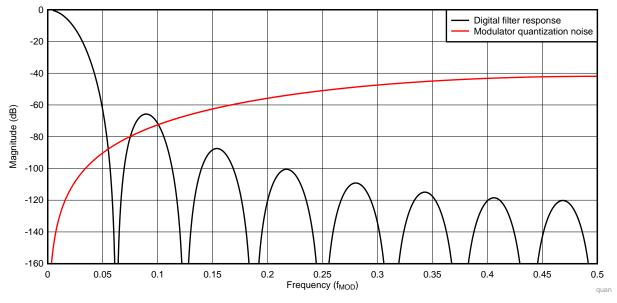
Figure 1. Spectrum of Delta-Sigma Quantization Noise and a Sinc Low-Pass Filter
