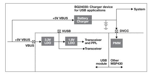
Figure 4. Power over USB can also be used as a primary source to charge batteries. This BQ2407x/3x family of chargers have been specifically designed for USB battery charging applications.
