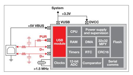
Figure 1. Integrating USB with the powerful performance and high integration of the MSP430 architecture creates the ideal microcontroller for implementing USB in embedded applications.
