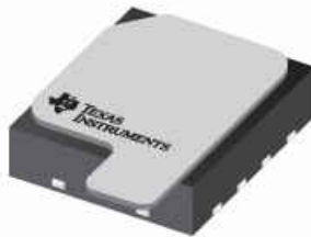
Figure 1-2. HDC3021 in a WSON Package
