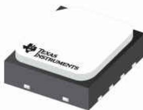
Figure 1-3. HDC3022 in a WSON Package
