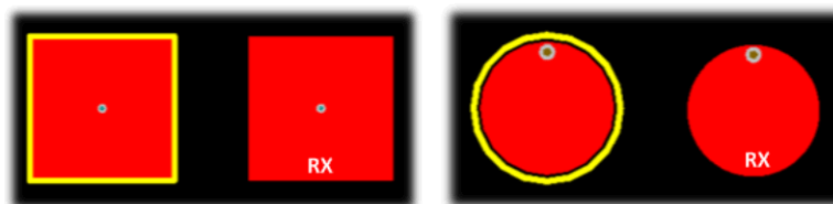
Figure 9. Button Shape for Self Capacitance
