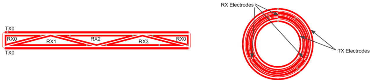
Figure 13. Mutual Capacitive Slider and Wheel
