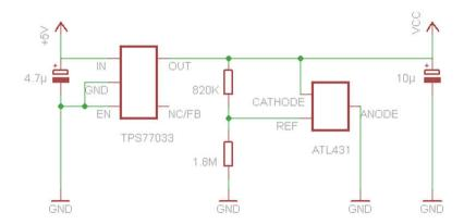
Figure 3-8. Schematic Example Using ATL431
