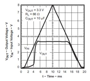
Figure 3-5. Power-Up and Power-Down Behavior of TPS715A
