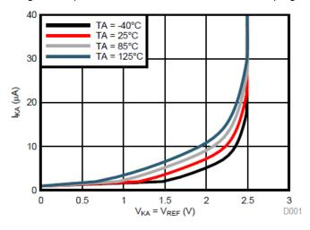
Figure 3-7. Cathode Current vs Cathode Voltage
