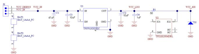
Figure 3-6. Alternative Solution Using a Zener Diode
