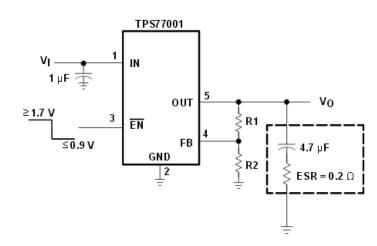
Figure 22. TPS77001 Adjustable LDO Regulator Programming
