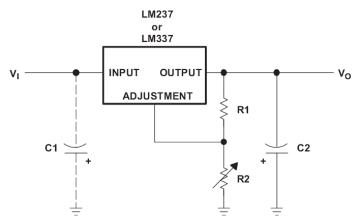
Figure 3. Adjustable Negative-Voltage Regulator
