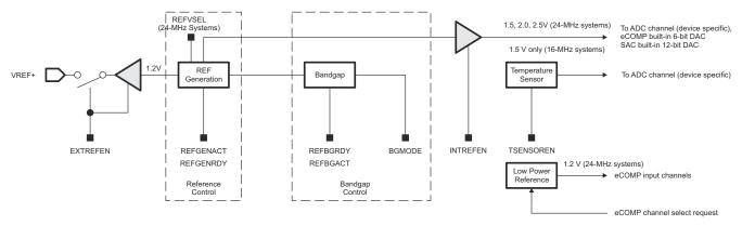
Figure 7-2. FR4xx Internal Reference Block Diagram
