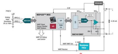
Figure 3: Field transmitter featuring HART<sup>®</sup> communications
