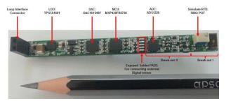
Figure 4: Current loop TI Design using the MSP430FR5738 MCU
