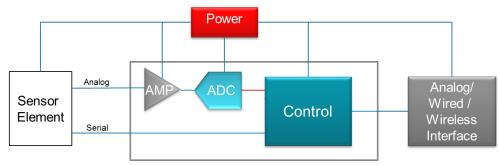
Figure 1: A typical industrial sensing system
