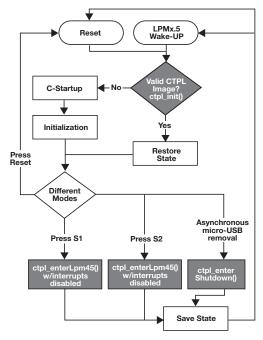
Figure 1: Flow of an Algorithm Leveraging Compute Through Power Loss
