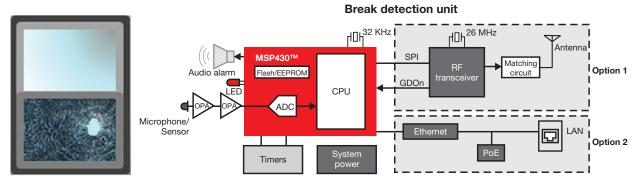
Figure 2: Sensors like glass-break detectors can be simple in implementation or utilize a more complex design requiring more processing capacity to increase detection accuracy.
