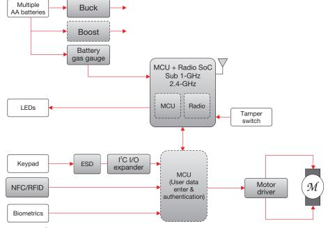
Figure 3: Some building automation equipment, like an electronic lock, employs a combination of mechanical and electronics. These designs require a low-power, flexible platform that can support different technologies, such as keypads, fingerprint readers, RFID cards and security tokens.
