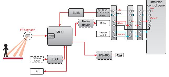
Figure 1: Sensors like **occupancy and motion detectors** operate primarily in a deep sleep, ultra-low power operating mode as they do not need to function until activity is sensed. Once an event is detected, these systems need to wake, process sensor data efficiently, act on the data and drop back into sleep or standby mode as quickly as possible to minimize energy consumption.
