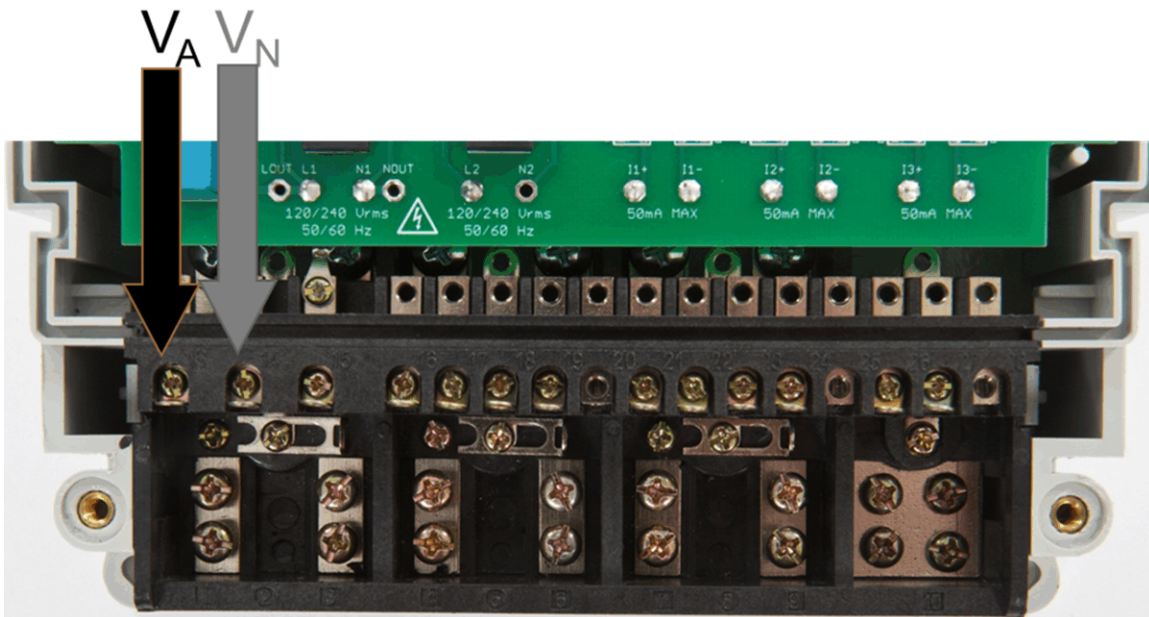
Figure 17. Top View of EVM with Test Setup Connections, Neutral-Monitoring and Common-Voltage
