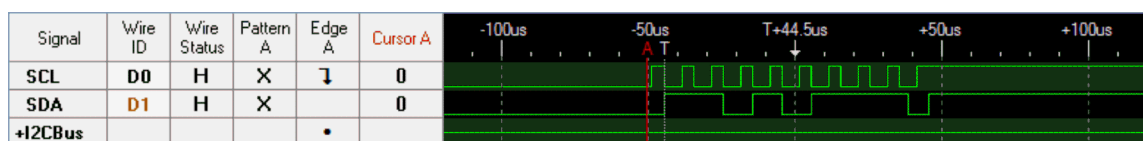
Figure 15. I 2 C Transaction for I2C_MASTER_CMD_BURST_RECEIVE_FINISH
