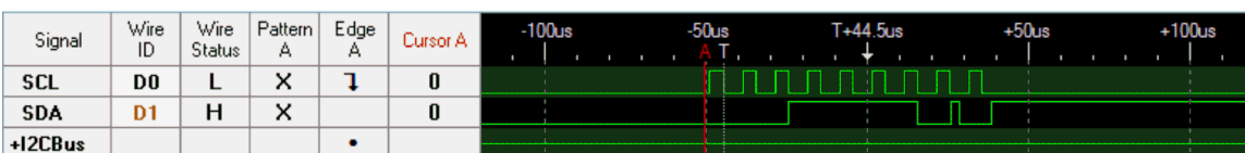
Figure 14. I 2 C Transaction for I2C_MASTER_CMD_BURST_RECEIVE_CONT
