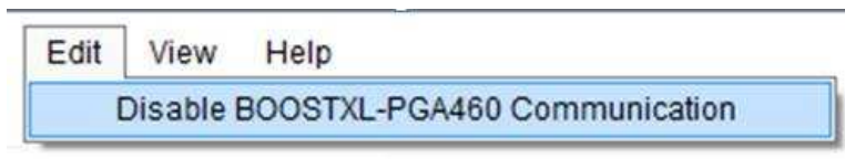
Figure 21. Disable Communication to PGA460 on BOOSTXL-PGA460 Motherboard
