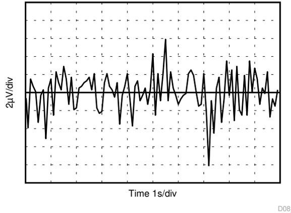
**Figure 6-2. REF3425 0.1Hz to 10Hz Noise**
